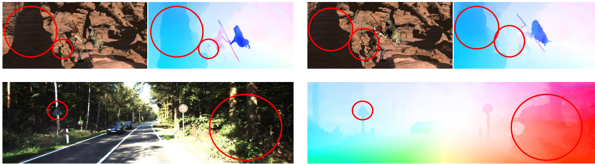
Fig. 11: Some failure cases and affected regions of our TransFlow under significant illumination changes and shadows. \circ highlights failure regions. See §4.4 for details.
